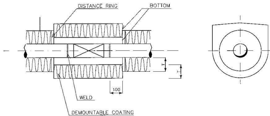
VALVE < Dn 80 COATING WITH SCREWS
