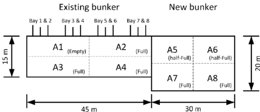
Total storage capacity with new bunker shall achieve at least 8 days compared to the existing 4 days of storage capacity at a waste treatment capacity of 44 ton/h. The new bunker shall be operationally divided into four areas, i.e. A5 to A8. In a situation with when bunker areas A7 and
