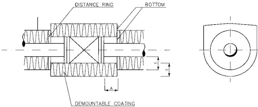
VALVE < Dn 80 COATING WITH SCREWS
